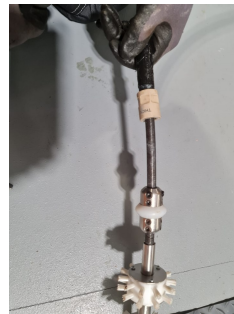
Leave a gap between the sleeve and the Twister of approximately 6mm (1/4").
