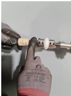
Leave a gap between the sleeve and the Twister of approximately 6mm (1/4").
