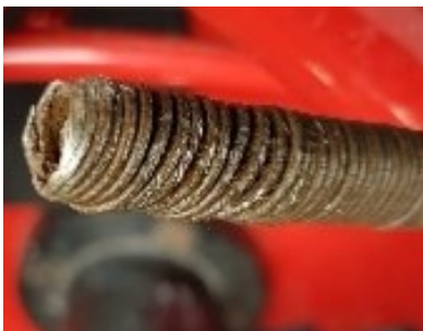
Damaged Shaft. Needs to be trimmed.
