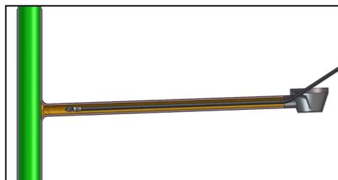
**Step 3.** Place a CCTV camera into lined pipe so that you will see how the work is progressing. **Never work blind!**
