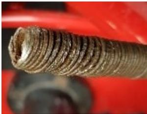
Damaged Shaft – needs to be trimmed back
