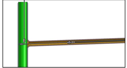
**Step 7.** Attach a larger Drill Head 3D Cutter to the shaft.
