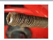
Damaged Shaft – needs to be trimmed back
