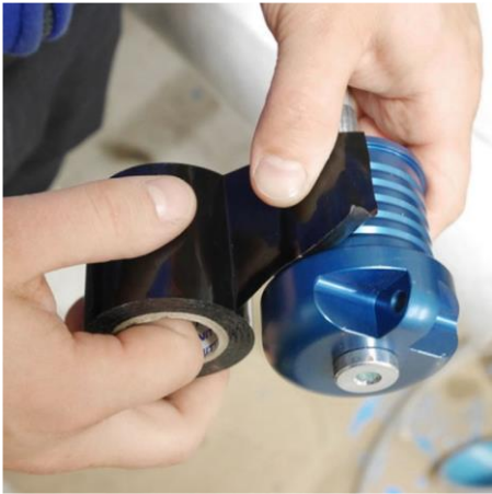
1. Tape the Packer heads with Nitto or Silicone tape
