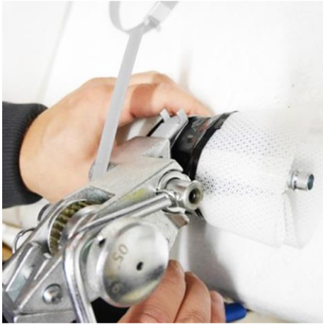
4. Tighten the steel strip to the bladder
